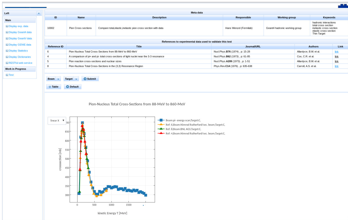
Figure 4. Display of a Geant4 simulation (blue squares) estimating the total cross section of \pi^- on a Carbon target as a function of kinetic energy. On the top we find information describing the Geant4 test and the publications from which the data for physics validation was extracted. The menus on the top of the graph are automatically created based on the contents of the database. In this case, one can select results based on target material (Pb, Cu, S, C, Au, Ag, Sn, Ca, Fe) and beam particle ( \pi^+ , \pi^- ). If there are more variables to choose from, then additional menus will be created. Each test comes with a set of defaults and one automatically gets the default plot when initially selecting a test. If the overlay option is selected, DoSSiER will search the database for any experimental results matching the meta-data of the test selection. In this case the search finds measurements from three different publications (orange, green, red curves) and overlays them on the simulation result.
