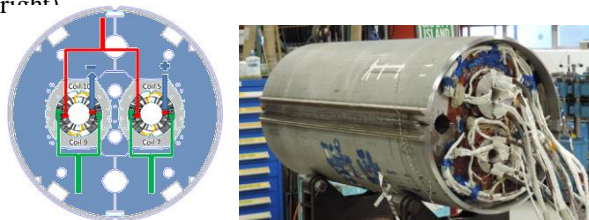
Figure 1: The coil electrical connection (left) and the assembled MBHDP01 cold mass before end plate welding and coil splicing (right).
