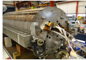
Figure 5: MBHSM01 mirror inside the bolt-on half-skin.
