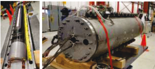
Figure 3: The 1 m long coil (left) and the single-aperture dipole cold mass MBHSP02 (right).
