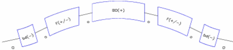
Fig. 4. A single lattice cell of the 50 Hz, 4 MW, 10 GeV, NFFAG proton driver ring.
