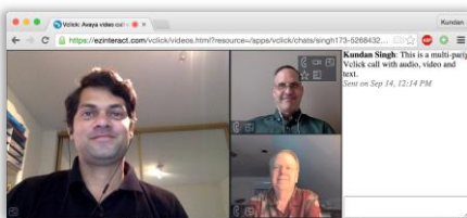
Fig.1. Screenshot of the Vclick conversation page in a 3-party call. Each video box or text chat is a separate widget with its own URL and runs in a separate iframe.
