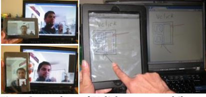
Fig.4. Screenshots of Vclick apps on mobile. (L) conversation apps with video on tablets. (R) a separate tablet is used to join the white-board app of the call where voice and video are on desktop.
