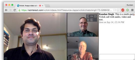
Figure 4. Conversation page in a three-party call with voice, video and text chat. The extension icon next to the address bar reflects the user’s presence or call state in that browser tab.
