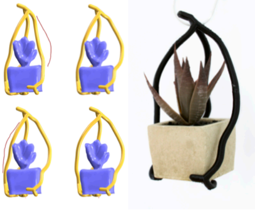
Fig. 9. Use of sketch modifications for a functional purpose. Top part of the planter holder is enlarged to be able to insert the planter. Left: Sketch modification steps, Right: 3D printed result with the inserted planter.
