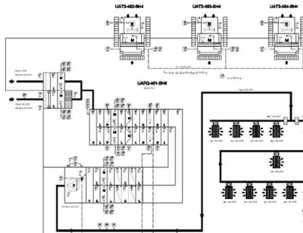
Figure 1: Example Process and Instrumentation Diagram (P&ID)
