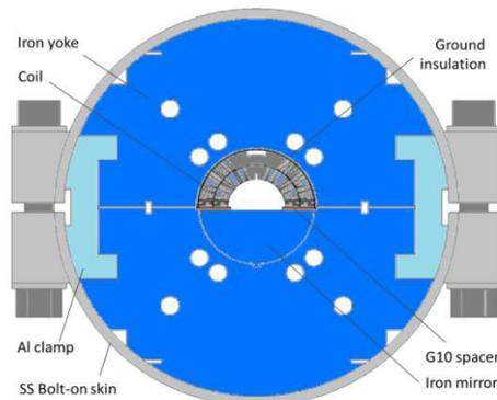
Figure 1: MBHSM01 dipole mirror cross-section.
