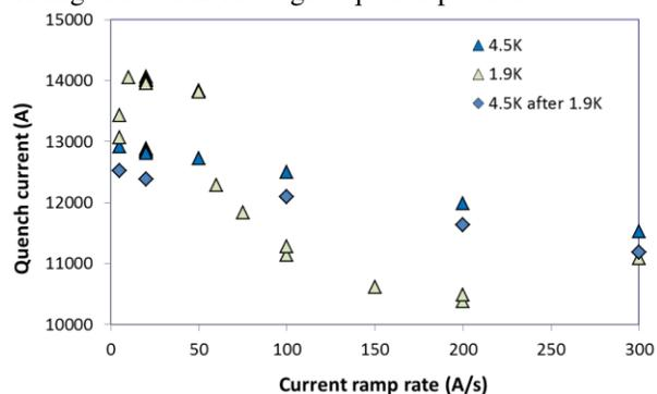
Figure 9: Ramp rate dependence of coil quench current.
