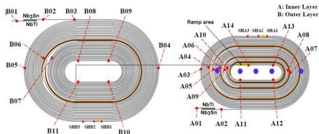
Figure 4: Voltage tap scheme in MBH08 coil.
