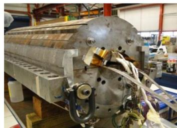
Figure 5: MBHSM01 mirror inside the bolt-on half-skin.
