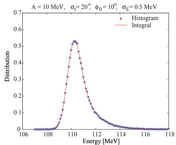
Figure 2: Energy distribution after the PETS for a beam with initial energy  $E_0 = 120$  MeV and maximum loss of  $A = 10$  MeV. Here the initial rms energy spread was taken to be 0.5 MeV. The blue dots are generated in a simulation the red line is the result of Eq. 11.
