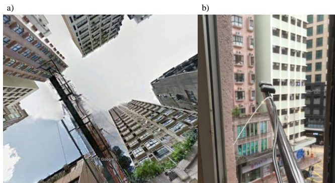
Fig. 2. a) denotes the environment of the multipath and NLOS data was collected and b) indicates the installment of the patch antenna.
