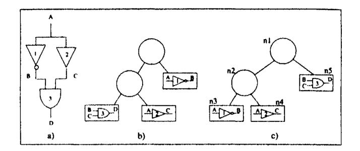
Figure 2: A device with two decomposition trees.
