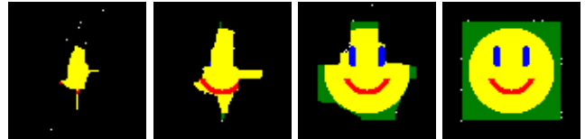
Figure 4: Snapshots of ten robots (white) building a structure of four block types (yellow, red, blue, green).
