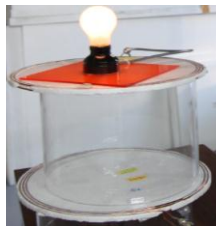
Fig. 1. Wireless power transfer using prototype resonators used in the experiments.
