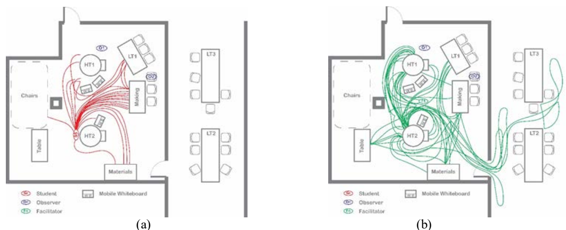
Figure 1. Spaghetti diagram showing the movements of Student 5 (a) and Facilitator 1 (b) during the activity
