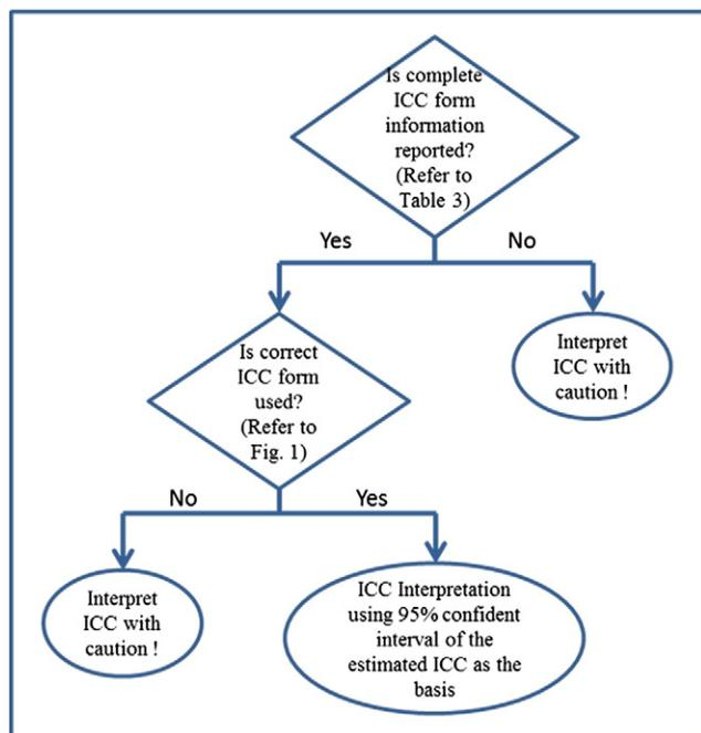
**Fig 3.** A flowchart showing readers how to interpret ICC in published studies. Values less than 0.5 are indicative of poor reliability, values between 0.5 and 0.75 indicate moderate reliability, values between 0.75 and 0.9 indicate good reliability, and values greater than 0.90 indicate excellent reliability.
