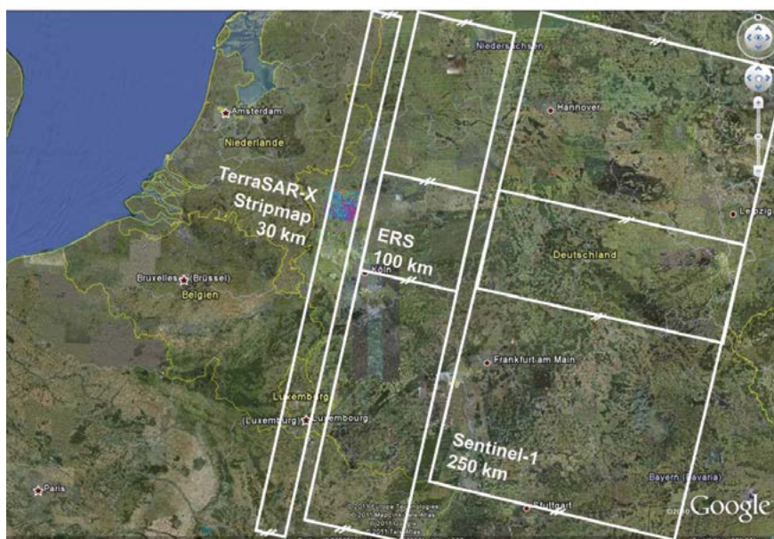
Figure 6. Single pass coverage of Sentinel-1, ERS and TerraSAR-X compared. (ESA)
