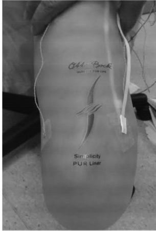
Fig. 1. Placement of the thermocouples on the lateral and medial side of residual limb skin and its corresponding positions on the liner of the transtibial amputee.
