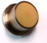
Figure 16: Sensor prototype with PEEK filler
