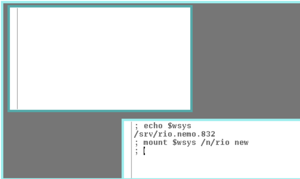
Figure 12.3: Mounting rio creates a new window. In this one, no shell is running.
