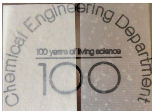
Figure 3. A comparison of the optical transparency of NFC and BC papers. Left: BC paper and right: NFC paper.
