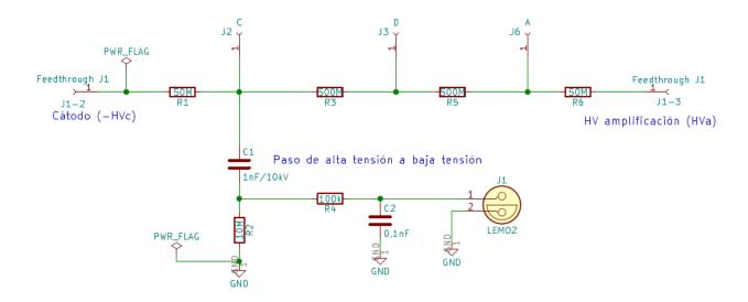
Fig. 2: Diagram of the cathode and the reading system.
