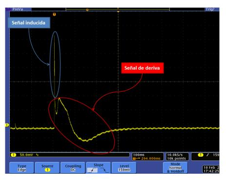
Fig. 3: Induction and drift signals produced at the needle and the cathode.
