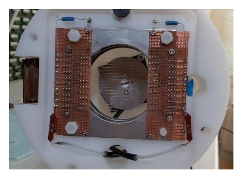
Fig. 1: Double grid cathode.
