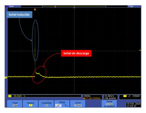
Fig. 4: Signal registered with the cathode at 0 V. The drift signal disappears and a discharge is visible.
