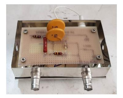
Fig. 6: High voltage pulse generator.
