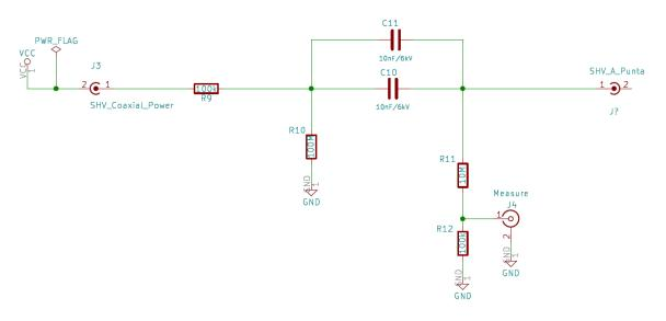
Fig. 5: Pulse generator circuit diagram.
