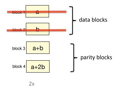
tolerates any two failures
