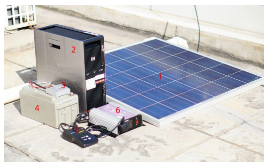
Figure 12: The system prototype: 1. solar panel, 2. workstation, 3. charge controller, 4. battery, 5. power meter and 6. inverter.
