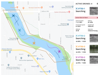
Figure 8: The user can mark an area on the map to define either a region or a point of interest to be targeted by the H2D directive.
