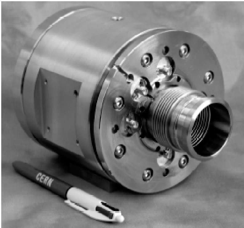
Figure 3: The IPU assembled. On the front there are four pick-up outputs and two calibration inputs.
