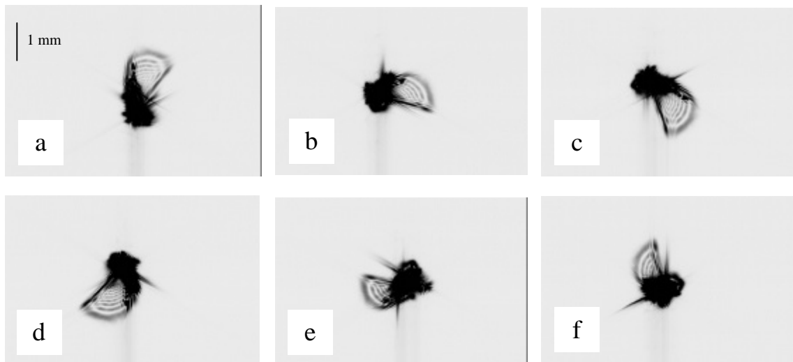
Fig. 4.65: Spot shape variation for mirror positions indicated in Fig. 4.32. The spot orientation corresponds to the orientation of the mirror on the holder, but also the spot shape changes. This proves small but not negligible influence of the holder on the spot size and shape.
