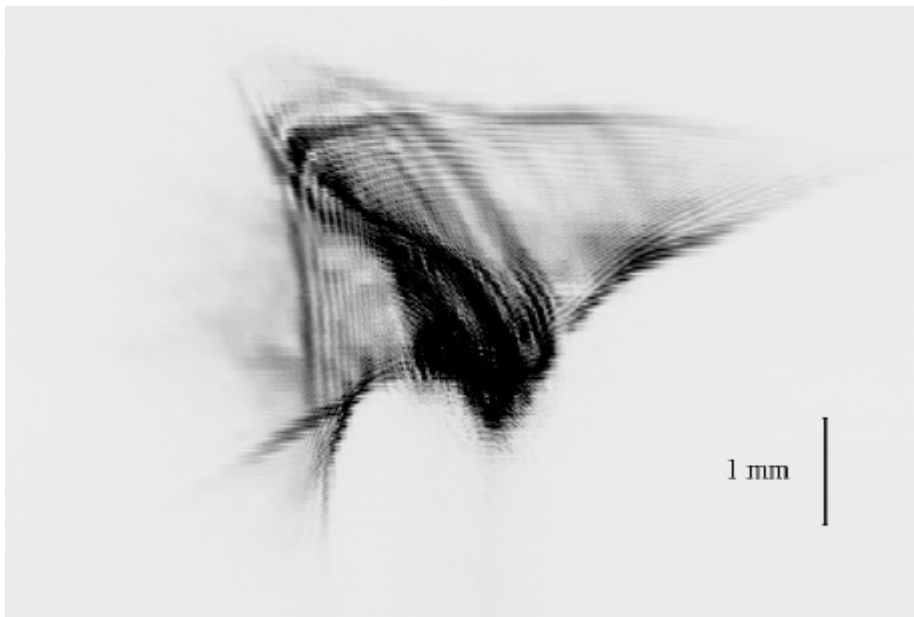
Fig. 4.7: Spot image from the circular prototype of the LHCb RICH 2 mirror with d = 400 mm, R = 7800 mm and t = 7.5 mm. 95 % of the reflected light was focussed inside a circle with diameter D = 3.4 mm.
