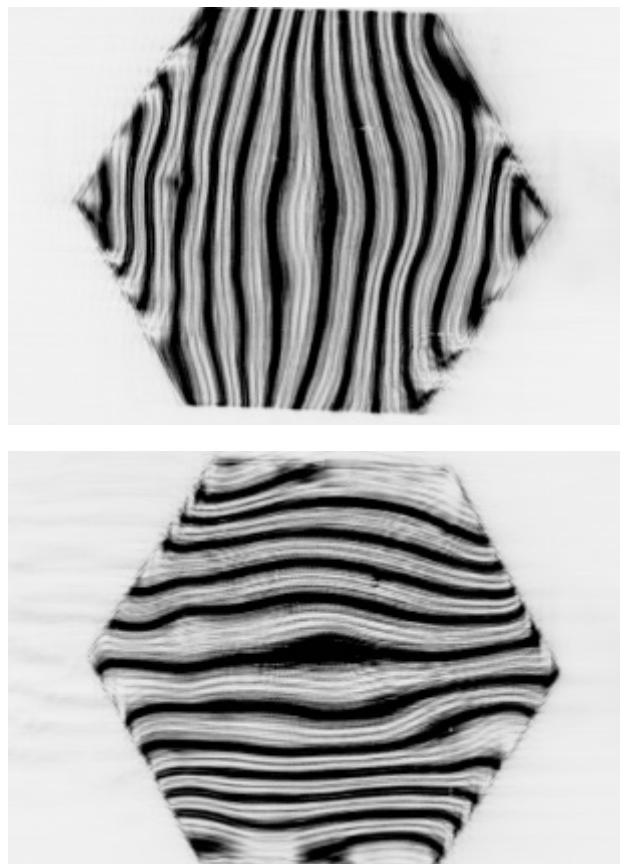
Fig. 4.15: Ronchigrams from the thin prototype of the LHCb RICH 2 mirror (thickness 4.5 mm, diagonal 502 mm, 95 % of reflected light focussed inside D = 1.66 mm). Deformed lines with varying thickness indicate distortions of the spherical shape.
