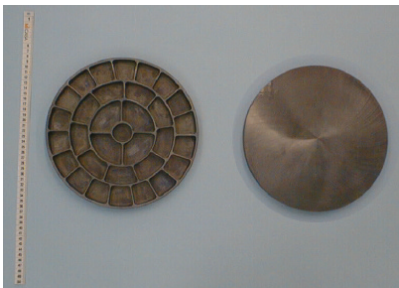
Fig. 4.71: The first Beryllium prototype. Left: back side with a structure of reinforcing ribs. Right: front side with a polished glass layer.
