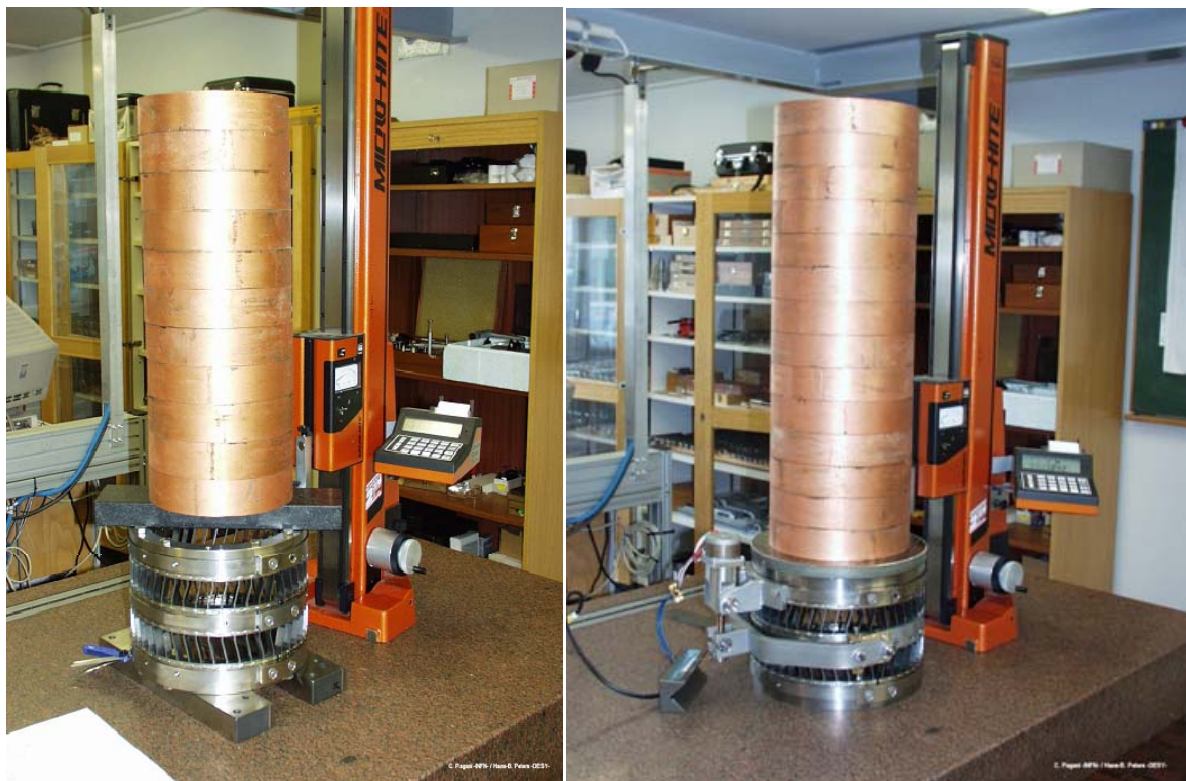
Figure 14: pictures of experimental compression tests on blade tuner, showing both the experimental configurations.
