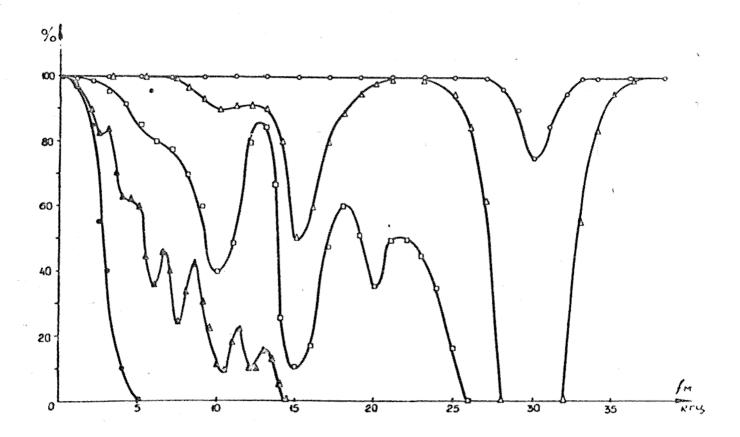
FIGURE 16: Dependence of the variable component of the photomultiplier current on the modulation frequency:  $o - \Delta f_M = 5 \text{ kHz}$ ;  $\Delta - \Delta f_M = 15 \text{ kHz}$ ;  $\Delta - \Delta f_M = 30 \text{ kHz}$ ;  $\Delta - \Delta f_M = 60 \text{ kHz}$ ;  $\Delta - \Delta f_M = 120 \text{ kHz}$ . Horizontal scale = kHz.
