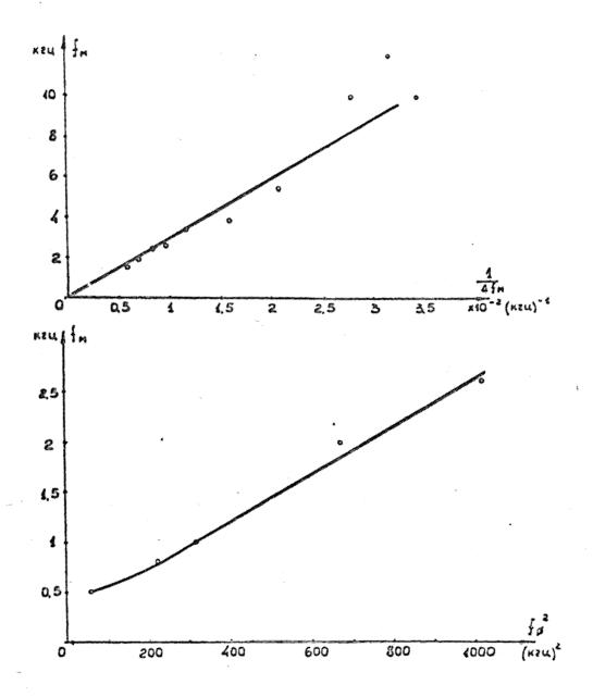
FIGURE 17: Dependence of the lower boundary of complete destruction of the RBPS on: a) the deviation ( $f_{\phi}$  = 34 kHz); b) the resonance power ( $\Delta f_{M}$  = 100 kHz). Vertical scale = kHz; horizontal scale = (kHz)<sup>-1</sup> and (kHz)<sup>2</sup>, respectively.
