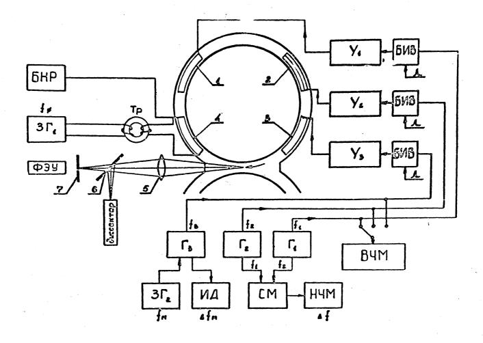
FIGURE 1: Diagram of the optical system of the BEP-1 storage ring and resonance-excitation system: 1, 3, 4 - buildup plates; 2 - buildup electrodes; 5 - lens; 6 - semitransparent mirror; 7 - diaphragm; 5 H P - nonresonant-buildup unit;  $3\Gamma_{1-2}$  - audio oscillator;  $\Gamma_{1-3}$  - HF oscillator;  $\Upsilon_{1-3}$  - power amplifier; 5 M B - pulsed on-off switching unit; B H M - HF frequency meter; H H M - LF frequency meter; C M - mixer; M A - deviation meter.
