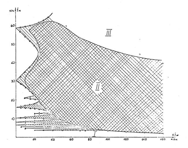
FIGURE 13: Stability diagram for periodic crossing through a resonance  $(f_{\phi} = 36 \text{ kHz})$ : I- slow ("adiabatic") crossing; II- stochastic region (o - complete destruction of the RBPS;  $\triangle$  - partial destruction of the RBPS); III- region of "modulation" resonances. Vertical and horizontal scale = kHz.
