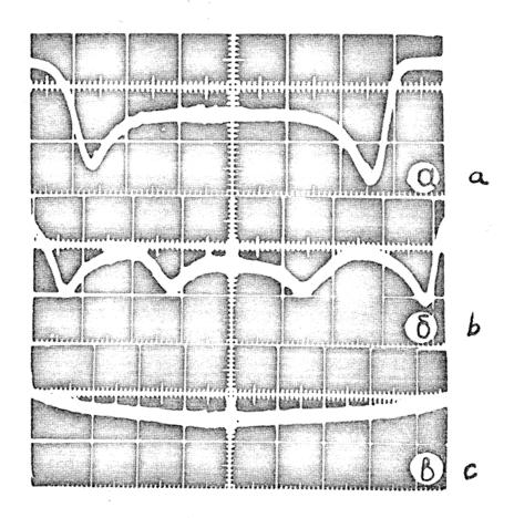
FIGURE 7: Oscillograms of the beam-density distribution with excitation of: a) a single resonance; b) two resonances m < 0.6; s = 1; c) two resonances m = 1; s = 1.
