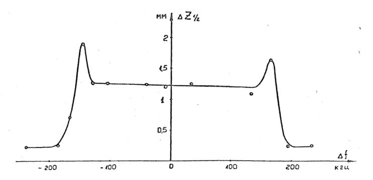
FIGURE 20: Dependence of the beam size on the buildup-frequency separation with respect to the exact resonance ( $f_{\phi}$  = 7 kHz,  $f_{M}$  = 5 kHz,  $\Delta f_{M}$  = 200 kHz). Vertical scale = mm; horizontal scale = kHz.
