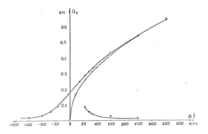
FIGURE 6: The equilibrium amplitude of the RBPS of a resonance of the vertical betatron oscillations as a function of the frequency separation. • - Ubuildup = 3 V; o - Ubuildup = 150 V.
