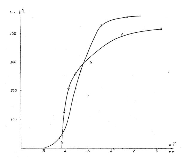
FIGURE 19: Dependence of the beam lifetime on the aperture with increasing beam size owing to: o - nonresonant buildup;  $\Delta$  - stochastic instability. Vertical scale = sec; horizontal scale = mm.
