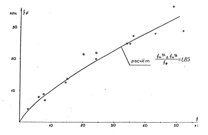
FIGURE 22: Dependence of the upper boundary of complete destruction of the RBPS on the resonance power ( $\Delta f_{M} = 100 \text{ kHz}$ ). Vertical scale = kHz; horizontal scale = kHz. Pacyët = calculation.
