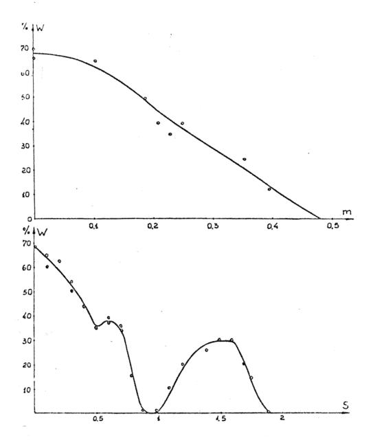
FIGURE 9: The probability of the particles' entrapment in RBPS $_1$  as a function of: a) the parameter m (s = 1); b) the parameter s (m = 0.4).
