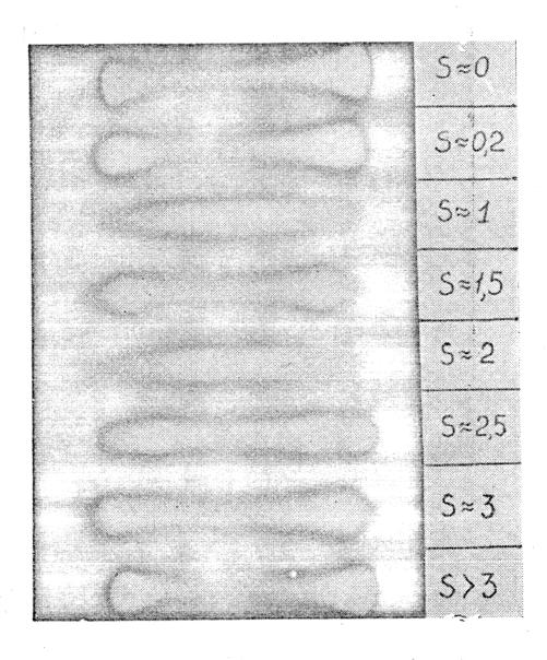
FIGURE 4:  $_{\rm Photographs}$  of the beam under the combined influence of two resonances of the vertical betatron oscillations as a function of the parameter s (m = 1).
