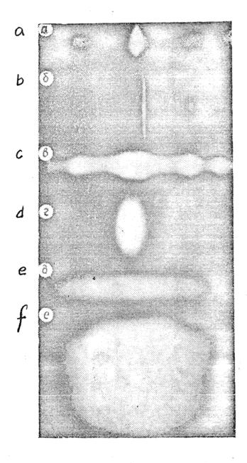
FIGURE 3: Photographs of a beam cross-section under the combined influence of two betatron-oscillation resonances: a), c) and e) two vertical; b) and f) a vertical and a radial; d) a radial and a sum.
