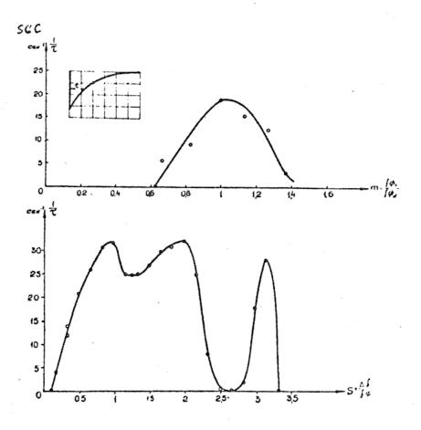
FIGURE 11: The time required for the particles to leave RBPS<sub>1</sub> when RBPS<sub>2</sub> is switched on, as a function of: a) the parameter m (s = 0.5); b) the parameter s (m = 1).
