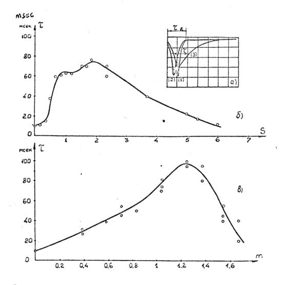
FIGURE 10: a) Oscillograms of the signal from the diaphragmed photomultiplier on passage of the beam through the amplitude region: 1- with no RBPS; 2- with one RBPS (RBPS<sub>1</sub>); 3- with two RBPS.
