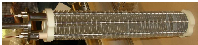
Fig. 2. Photograph of the inside of an ionization chamber. The stack of aluminum electrodes with the insulator ceramics at both ends can be seen.
