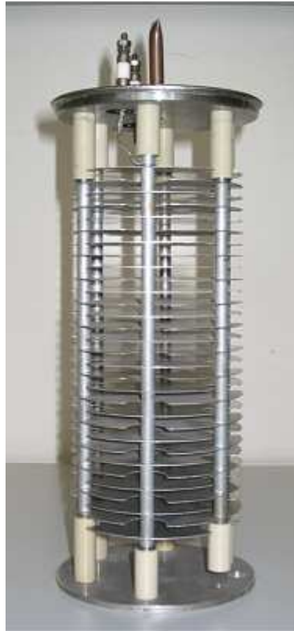
Figure 6.1. One of the ionization chambers that will be placed around the LHC ring in order to monitor the beam losses.
