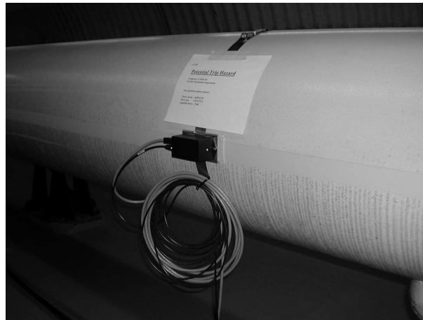
Figure 7.4. A photo of a PIN diode mounted on the outside of the RHIC cryostat.
