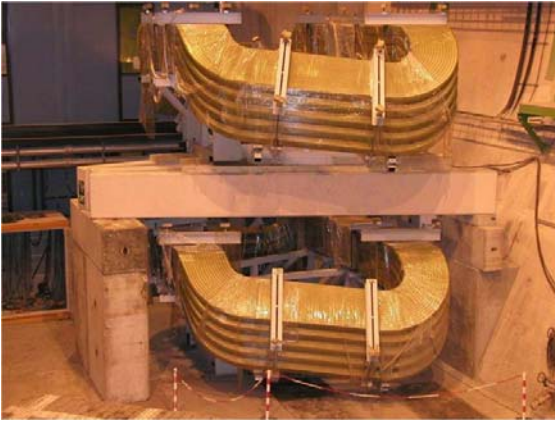
Figure 4.24: The two LHCb magnet trapezoidal coils.
