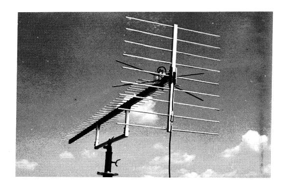
Fig. 4  $$5\lambda$$  37-element antenna with full-wave dipole feed
