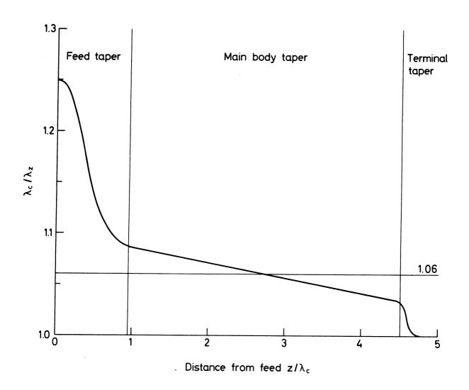
Fig. 1  $\frac{\text{Target phase velocity ratio distribution along slow-wave structure}}{\lambda_{\text{C}} = \text{free space wavelength}} \qquad \qquad \lambda_{\text{Z}} = \text{surface wavelength}}$
