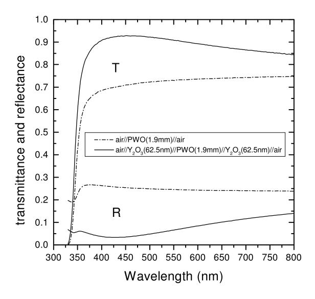
**Fig. 11:** transmittance and reflectance, at normal incidence, of the uncoated and coated PWO test piece. The experimental curves are well reproduced by assuming the films perfectly transparent (k=0), 62.5 nm thick and with the refractive index of a material composed by 76% in volume of Y<sub>2</sub>O<sub>3</sub> [7] and 24% of air, computed according to the effective medium approximation [9].
