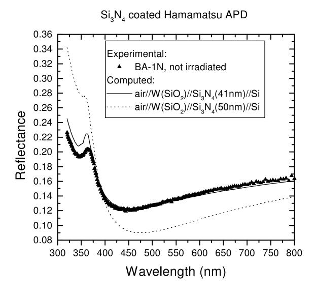
Fig. 7: reflectance of the  $Si_3N_4$  coated "BA1N" Hamamatsu APD compared with the computed reflectance based on the model "air//W(SiO<sub>2</sub>)//Si<sub>3</sub>N<sub>4</sub>(41nm)//Si". The effect of the  $Si_3N_4$  antireflection coating is more effective in the 400-520 nm range when the coating thickness is about 50 nm.
