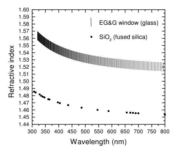
**Fig. 3:** experimentally determined refractive index of the EG&G APD window compared with the one of the SiO<sub>2</sub> (fused silica) [5] which, as discussed in the text, is assigned to the EG&G transparent glue (TG). In the same wavelength range, the extinction coefficient of the glass window is  $k < 1 \ 10^{-6}$ .
