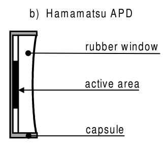
**Fig. 1:** section of APD's produced by EG&G and Hamamatsu. In both devices the Si wafer is enclosed in a capsule and covered with a transparent window. In the EG&G APD (Fig. 1a) the window is sealed to the capsule with some transparent glue. The Hamamatsu (Fig.1b) adopts a rubber window which completely fills the capsule-room and cover the Si surface together with the electric contacts (not reported in the figure).
