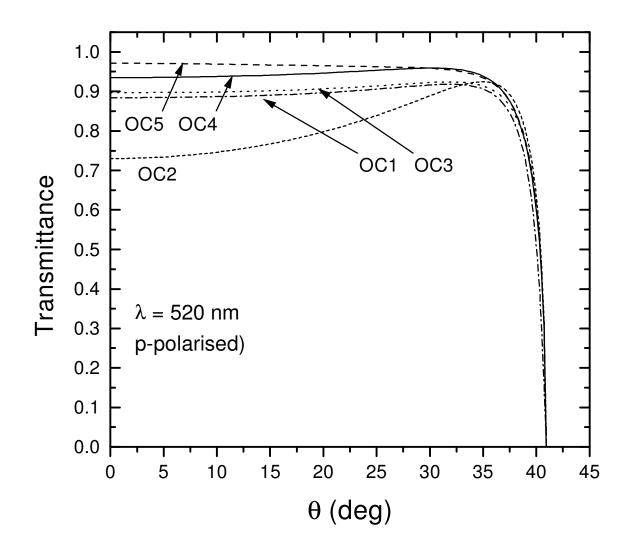
**Fig. 14d:** computed *p*-polarised transmittance, from the PWO to the Si, versus the incidence angle at 520nm for:
