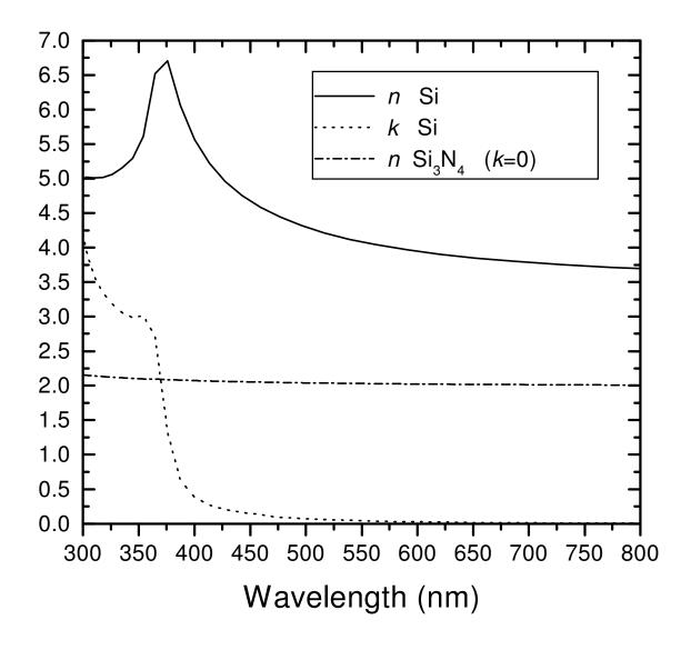
Fig. 5a: complex refractive indexes of Si and  $Si_3N_4$  [5].
