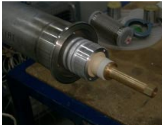
Figure 2: The prototype system. The left photograph shows the complete setup, the right photograph the end of one of the cylindrical vacuum tanks with an inserted MDT.
