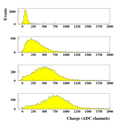
Figure 4: Charge distributions at 8.6 KV, 8.8 KV, 9.0 KV and 9.2 KV.
