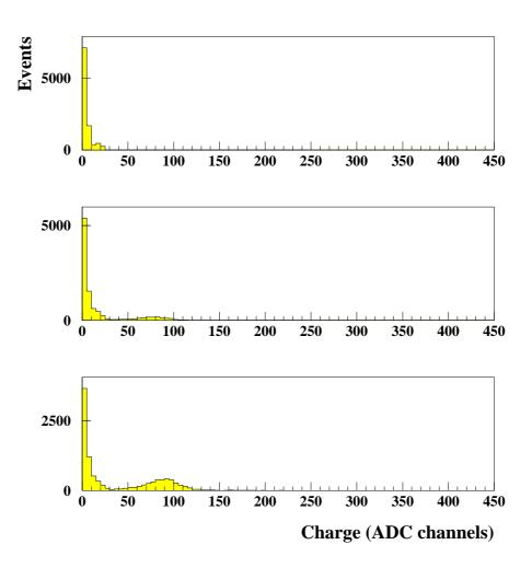
Figure 5: Charge distributions (without signal amplification) at 9.0 KV, 9.4 KV and 9.6 KV.
