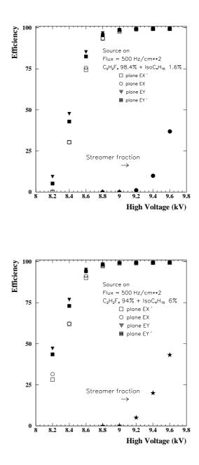
Figure 1: Efficiency and streamer fraction vs high voltage for two different gas mixture.
