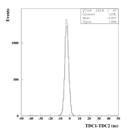
Figure 2: Time of flight between two RPC chambers at 9.0 KV.
