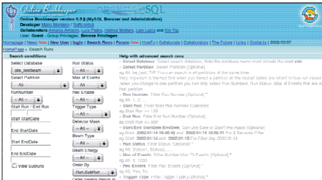
Fig. 4 The Online Bookkeeper graphical user interface to browse and append operational information and configuration description.
