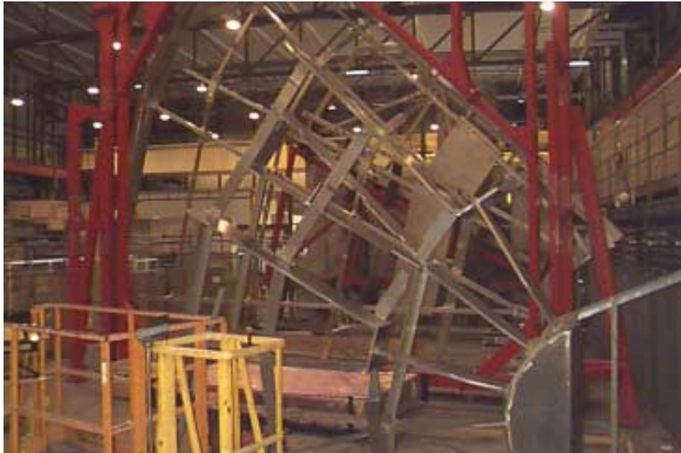
Figure 2: The three end-cap support structure EI, EM and EO as seen from the beam. The two phantom chambers installed on EO frame are also visible.
