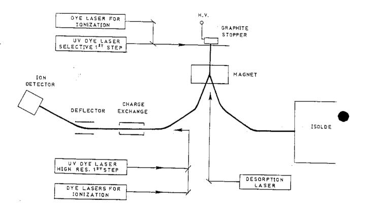
Scheme of the experiment. The upper laser system is used for desorption and first ionization. The lower system with high resolution is used to ionize the neutral fast beam in the collinear section.
