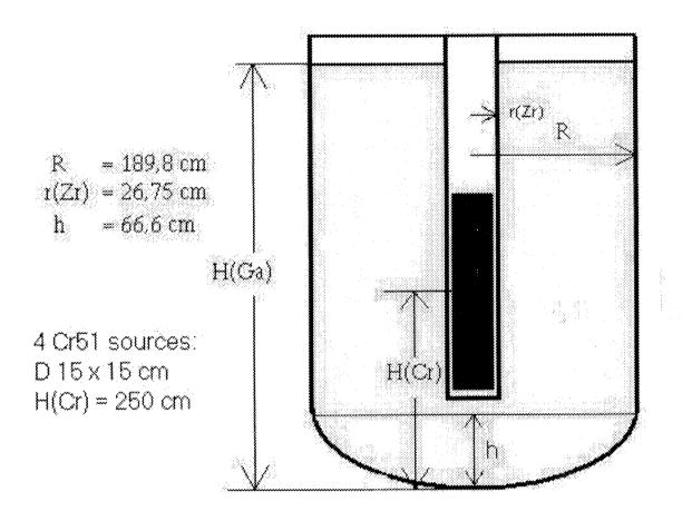
Fig.3. Geometry of new GALLEX calibration experiment.
