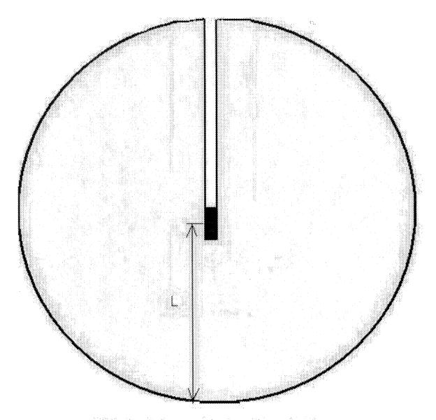
R(Ga) = 128 cm, Zr tube: D10 x 156 cm; Three 51Cr sources with W-shielding: D 8 x (3 x 14) cm L = 125 cm
