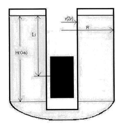
Fig.6. Geometry of new SAGE calibration experiment with single GALLEX source.
