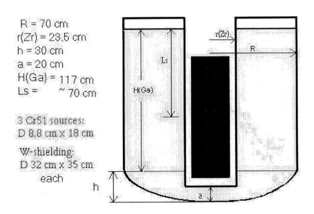
Fig.7. Geometry of new SAGE calibration experiment with composite GALLEX source.
