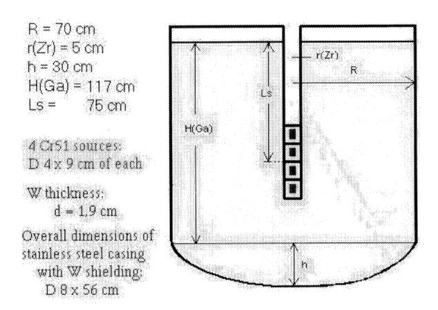
Fig.5. Geometry of new SAGE calibration experiment (with SAGE's composite source).
