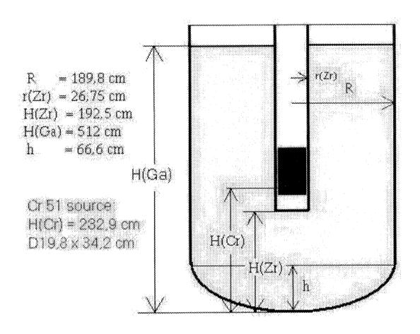
Fig.2. Geometry of GALLEX calibration experiment(s).
