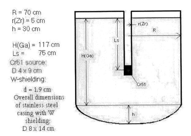
Fig.4. Geometry of SAGE calibration experiment.
