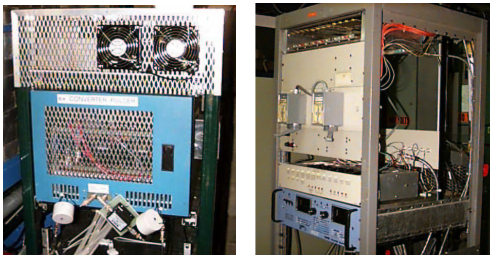
FIGURE 4.5: Pulser (left) and power supply with interlocks (right). RMS 600-8-2-D from LAMBDA EMI is used as a power supply.
