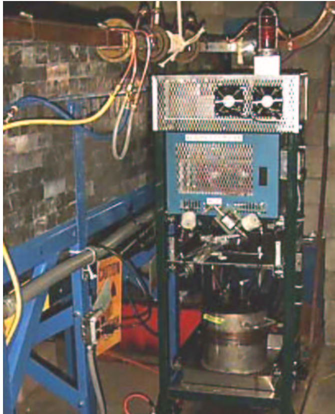
FIGURE 5.2: Pulser unit located in front of the converter cave. Section #4 is located at the left, behind the lead shield. Electron beam is running from the left side of the picture.
