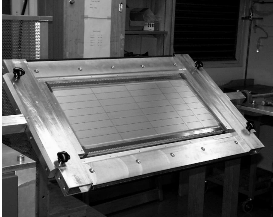
Figure 52 Wiring of a panel mounted to the aluminium frame.
