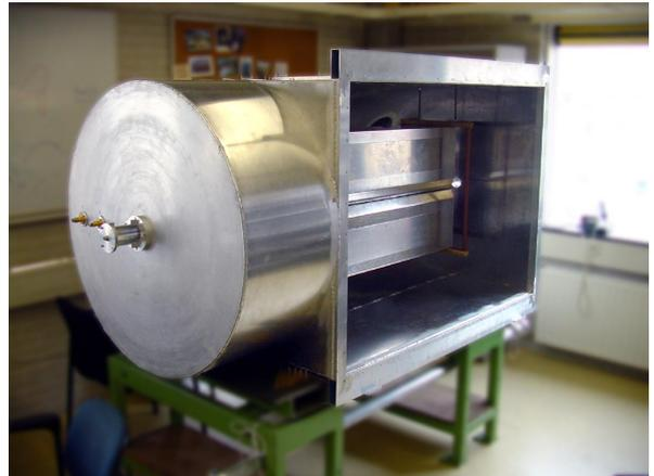
Figure 2.46: Full scale model of the VELO structure for RF tests.
