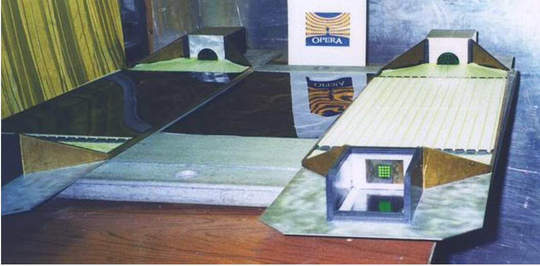
Figure 151: Prototype scintillator strip modules at the assembly site.
