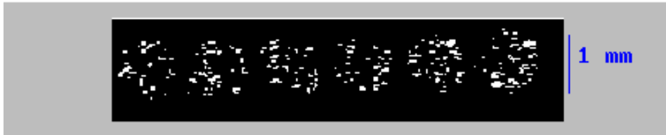
Figure 159: Typical image from the EBCCD, showing the single photoelectron signal from six WLS fibres for through-going mip .
