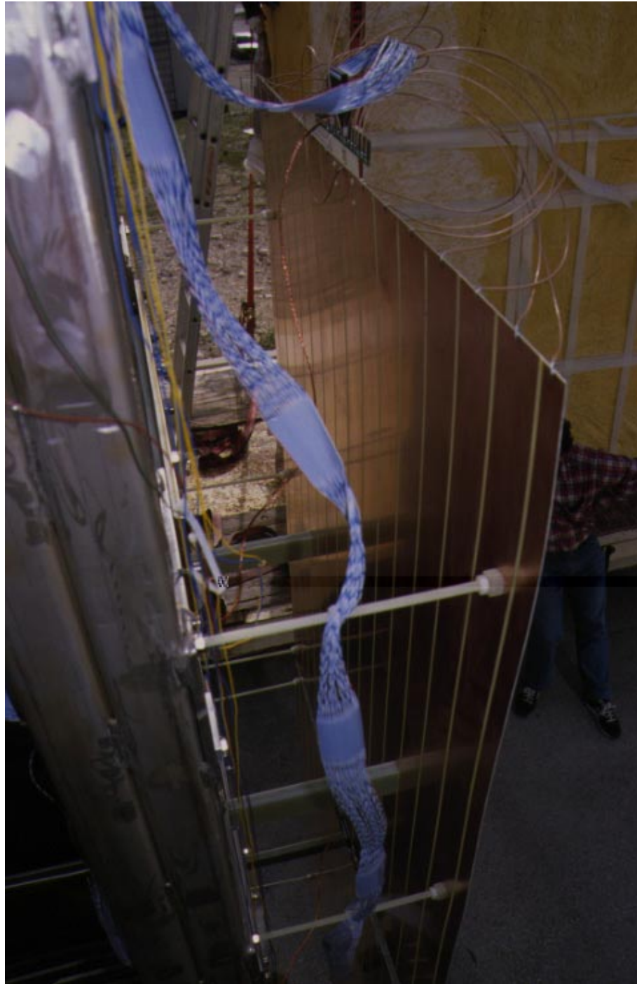
Figure 5.1: The planes of pads mounted onto the 10m^3 wire chamber frame. Connections and the signal flat cable are also visible. The distance between the plane and the mechanical frame is about 30 cm
