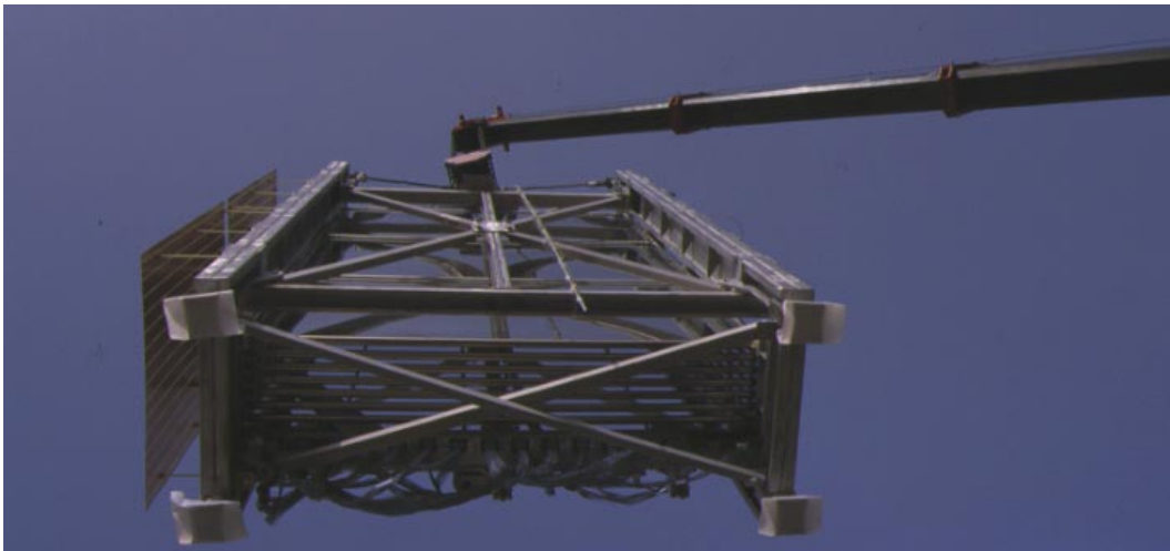
Figure 5.2: The inner detector during the insertion into the 10m 3 cryostat. The two planes of calorimetric pads are visible at the left-hand side of the wire chamber mechanical structure.
