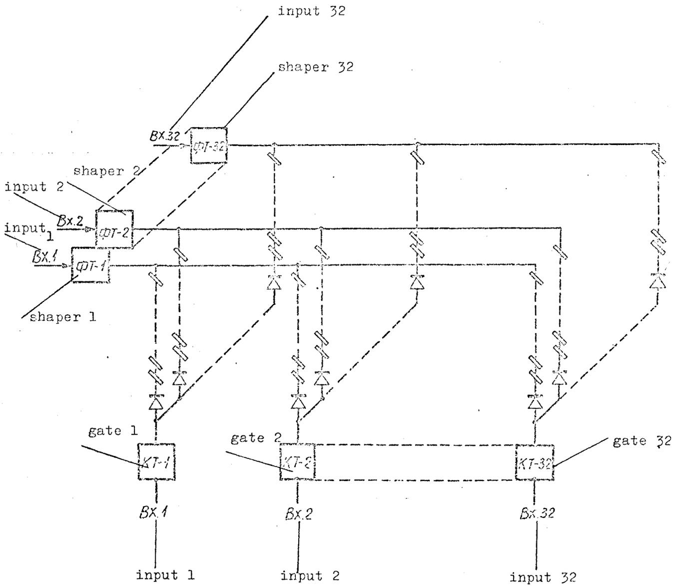
Fig. 3 Diagram of connections between current shapers, gates and matrices.
