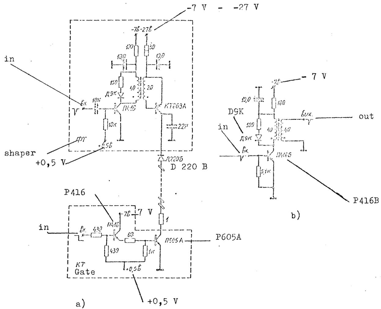
Fig. 2 a) current shaper and gate circuit;
