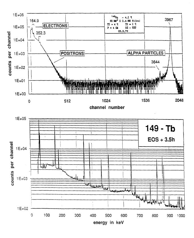
Fig.3 Spectra of particles (e<sup>-</sup>, β<sup>+</sup> and α) (upper part) and gamma rays (lower part) emitted from mass-separated and chemically purified <sup>149</sup>Tb samples 4 and 3.5 h respectively after end of separation. The spectra were recorded using a 80 mm<sup>2</sup> x 0.4mm Si(Au) surface barrier detector (upper part) and a 80 cm<sup>3</sup> HP-Ge-detector (lower part)
