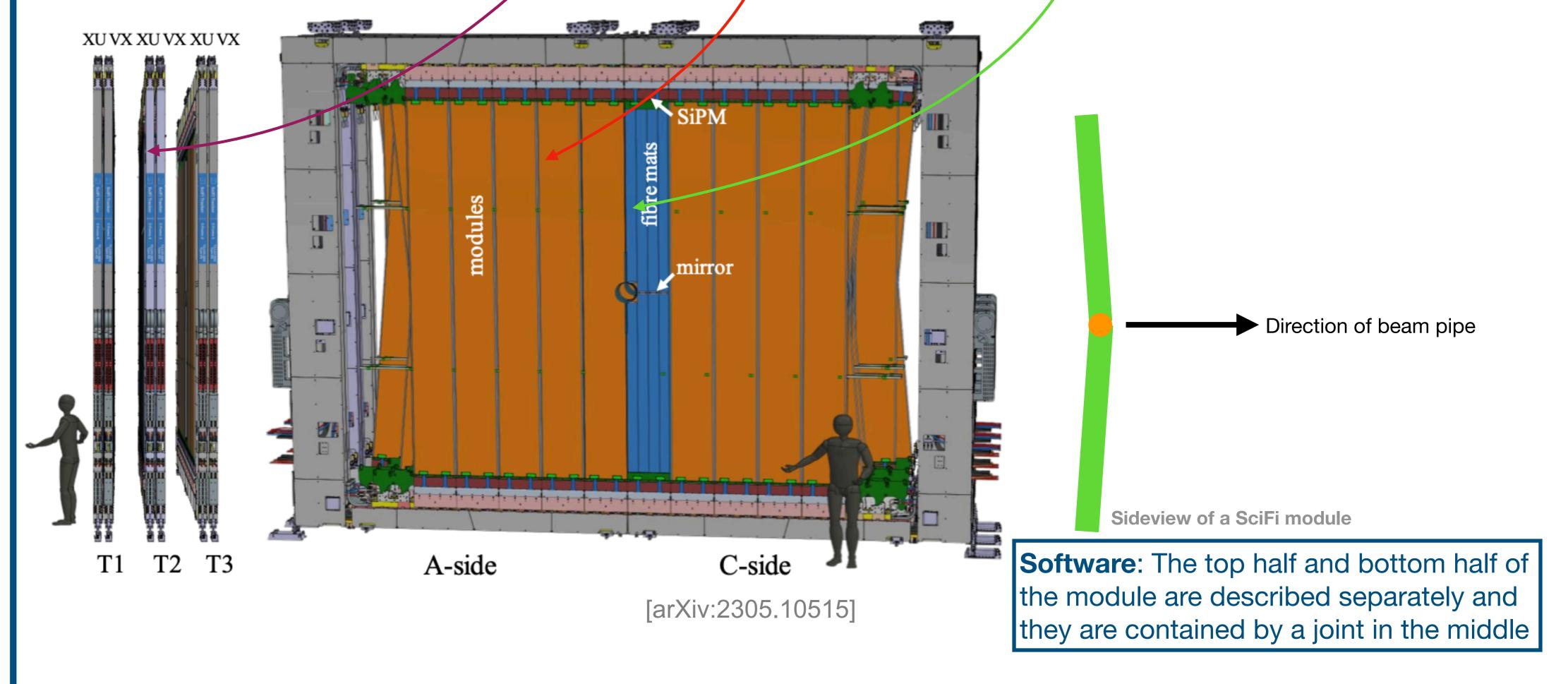
The SciFi modules are slightly bent around x-axis which the alignment has to account for
