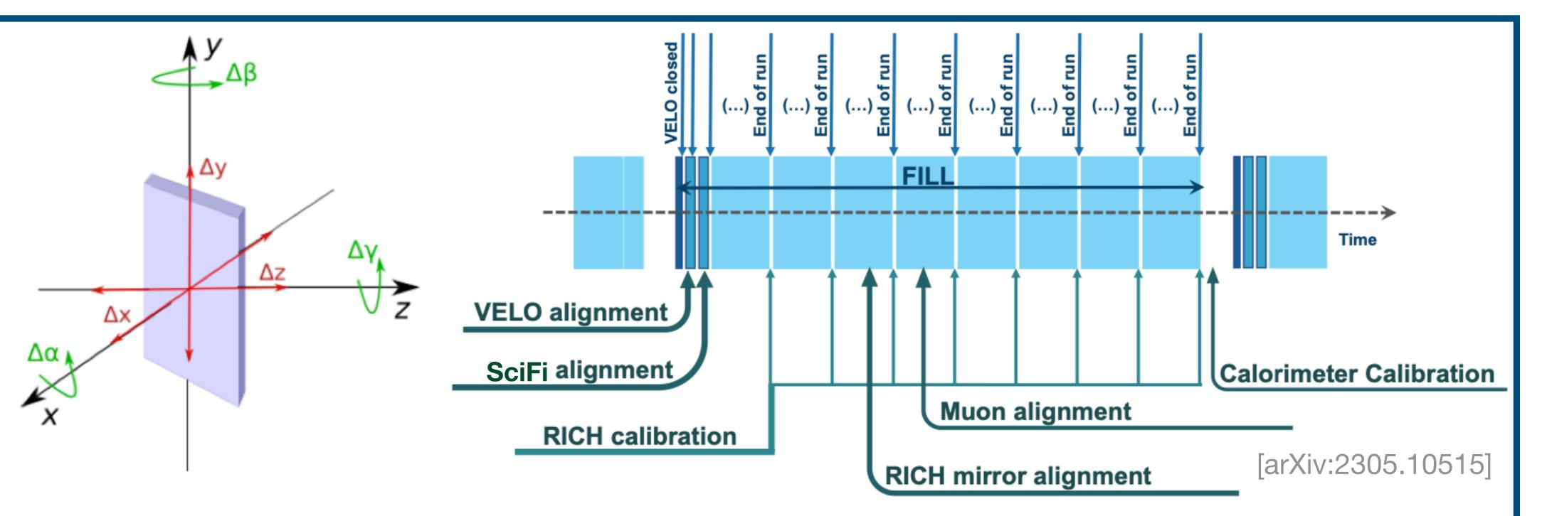
Alignment constants: transformations such as translations in and rotations of the detector components around the x, y and z axis Minimisation of the global track  $\chi^2$  yields optimal alignment constants  $x_i \rightarrow Update$  the alignment constants if they yield better performance
